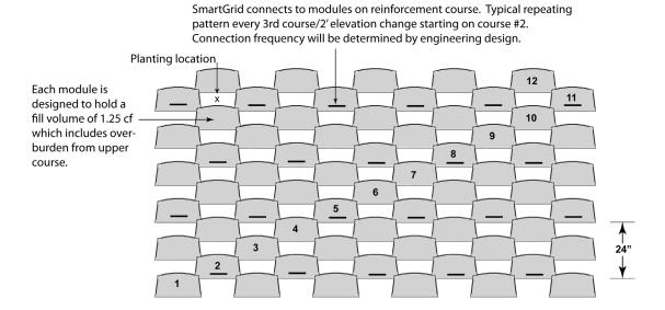
**Note:** Because GreenWay Wall Systems require batter between 20 and 40 degrees from vertical, installations impose a minimum footprint of 2.91" per course plus 15" for the length of the top module. A 12' tall wall at 70 degrees, will have a footprint of 5.37' as measured from the face of course #1 to the rear of course #18.
