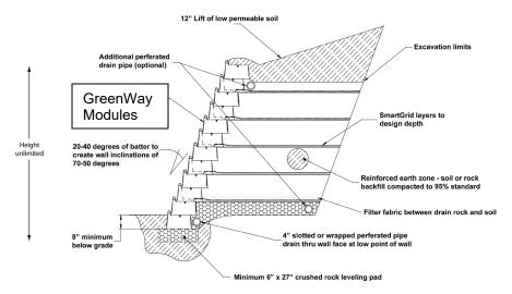
GreenWay batter enables design of greater wall height construction before reinforcement is required. Where reinforcement is required, GreenWay system includes a true mechanical connection through the module itself (no need for additional pins, rods, pipes, or other means of attachment) creating high connection values regardless of wall height. Wall design employs the same engineering protocols as any segmented retaining wall or slope stabilization.
