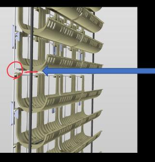
At the junction of the upper and lower kits, cut off the hose fittings and the end caps. Then connect the supply lines on both sides with the supplied 1/2" connector fittings
