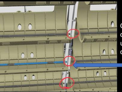
Cut off end ¼" end caps and connect using the ¼" connector fittings
